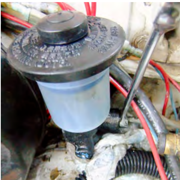
The hard line connection cracked open to allow fluid and air to drain out.
