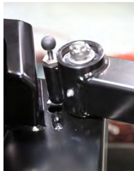
The spindle and safety pin mechanism.
